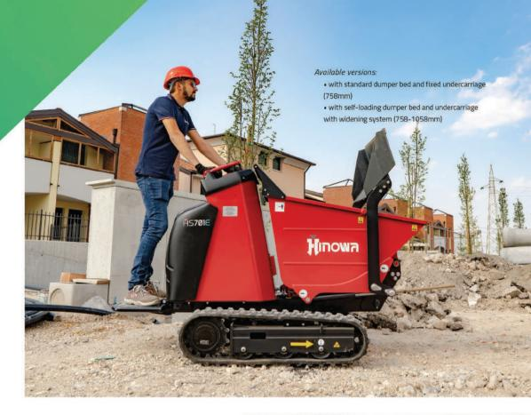
Elevated protection level of the traction motors used (P67 – 6=powder, 7=water). This high protection level is obtained by using innovating electric Internal Permanent Magnet traction motors instead of the traditional hydraulic ones, and it even allows to cross water bodies with the tracks.
