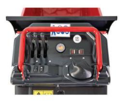
New control panel for an easy and safe use, with ergonomic joysticks and enabling button to prevent the operator from making accidental movements and with two available speeds: "ecomode" for uneven surfaces and energy saving, "power" for flat surfaces.
